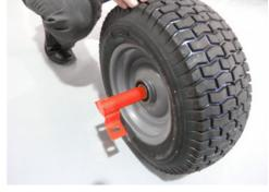
**Step 17.**Slide the wheel supports (12) on both sides of the shaft.
