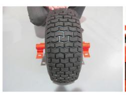
Place wheel assembly on top of the handles (5) and secure with S3 bolts.
